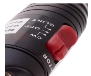
Fig. 4 Three modes of visual fault locator switch
