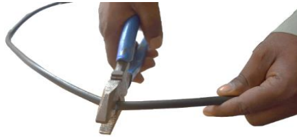
Fig. 2 Breaking damaged fibre using plier
