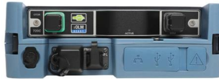
Fig. 1 Ports of optical time domain reflectometer
