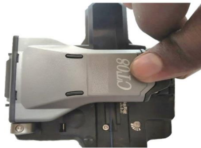
Fig. 3 Closing the cap of cleaver
