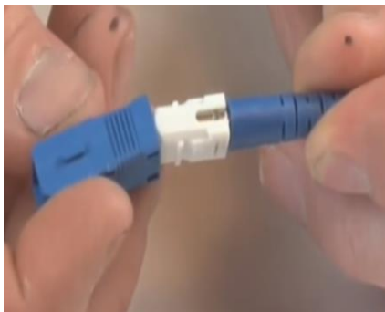
Fig. 6 Connecting outer housing to the inner body
