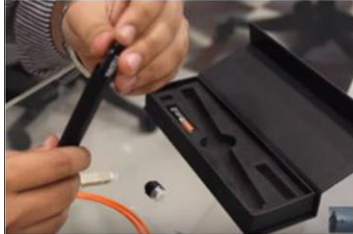
Fig. 3 Insertion of batteries inside the visual fault locator
