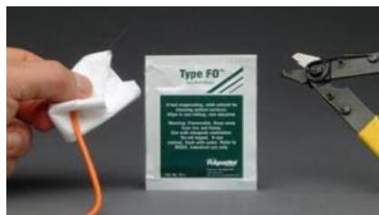
Fig. 2 Cleaning the optical fibre using tissue paper
