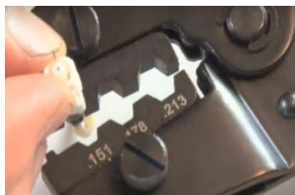
Fig. 5 Crimping using the crimper
