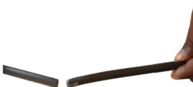
Fig. 2 Two ends of fibre cable which is to be splice
