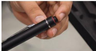
Fig. 4 Pressing of the button of visual fault indicator
