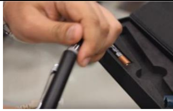
Fig. 2 Opening of the upper lid of the visual fault locator
