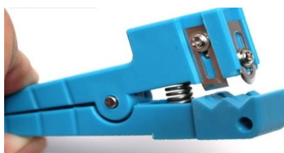
Fig. 1 Open the buffer tube cutter
