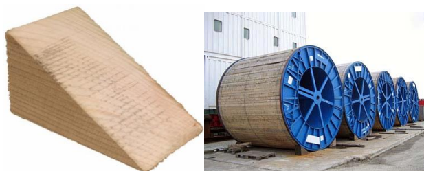
Fig. 3.3 (a) Wooden wedge (b) Wedge is placed to block cable drum
