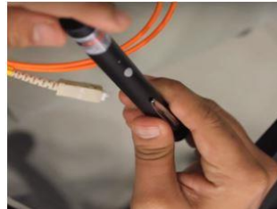
Fig. 5 Opening of the other end of the cap of visual fault locator
