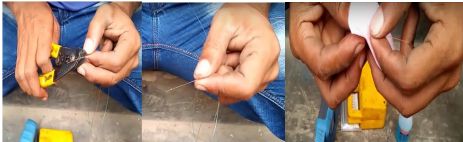
Fig. 7 (a) Stripping the buffer of OFC using optical fibre stripper, (b) Stripped fibre, (c) Cleaning the cladding using tissue paper
