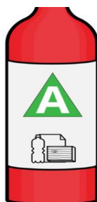
Fig. 1.20 Class A type fire extinguisher
