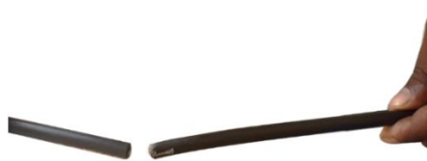
Fig. 3 Two ends of fibre cable which is to be splice
