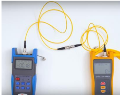
Fig. 5 Reading in the optical power meter
