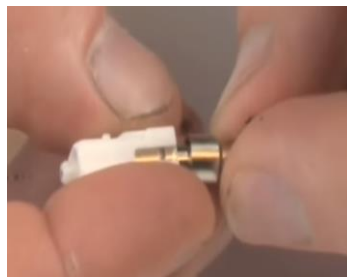
Fig. 4 Inserting stripped fibre inside a ferrule
