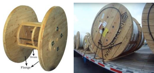
Fig.3.4 Drums are correctly placed on the truck
