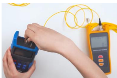
Fig. 2 Connecting the reference cord to the optical power meter and optical light source
