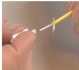
Fig. 3 Inserting the bare fibre inside the ferrule
