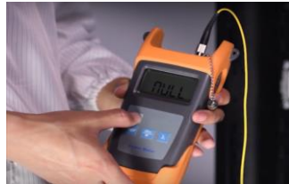
Fig. 2 OFC connected in optical power meter
