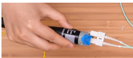
Fig. 2 SC-connector connected to the VFL
