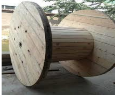
Fig. 3.19 Cable drum placed on hard and flat surface
