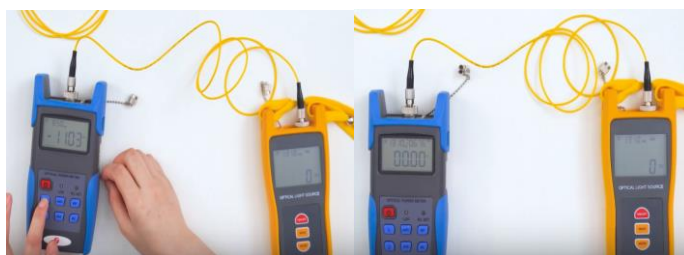
Fig. 3 Setting up the optical power meter and light source
