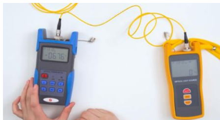
Fig. 3 Optical power meter with light source
