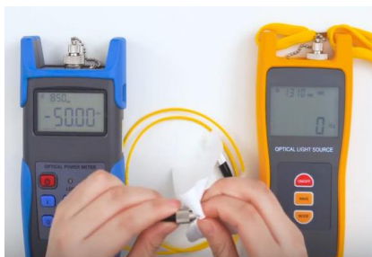
Fig. 1 Clean the ends of reference cord
