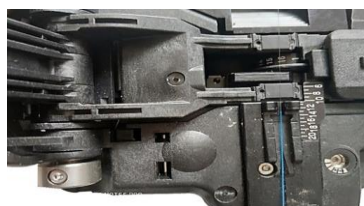
Fig. 2 Fibre placed in the slot of precision cleaver
