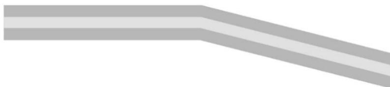
Fig. 2.9 Splice loss due to Axial run-out
