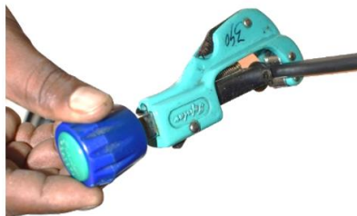
Fig. 4 Working of round cutter on the fibre
