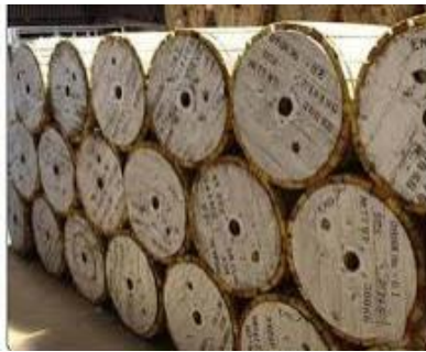
Fig. 3.18 (a) Cable drums are placed in an open area (b) Cable drums are placed in the shaded area (relevant Figure)
