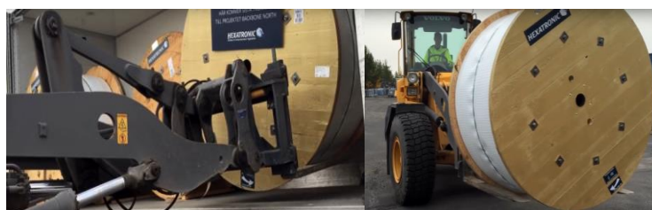
Fig. 3.10 (a) & (b) Forklift lifting cable drum
