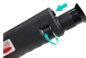
Fig. 3 Adjusting the focus control of the microscope
