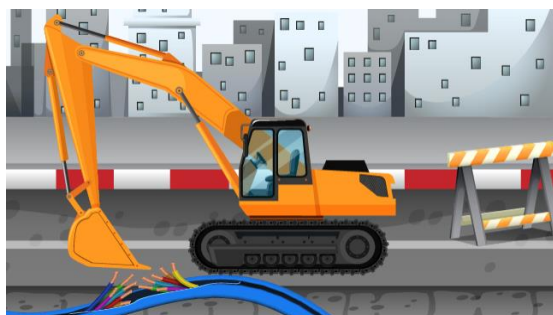
Fig. 2.6 Damage of the fibre cable due to construction
