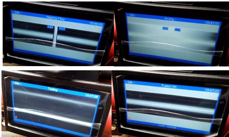
Fig. 9 Display unit shows the splicing operation going inside the fusion splice machine
