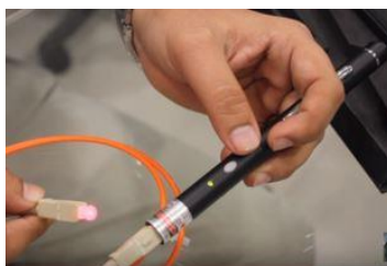
Fig. 9 Checking of the light passage through the fibre
