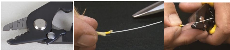
Fig. 1 (a) Three slots of optical fibre stripper (b) Buffer layers of OFC (c) Stripped fibre is placed in middle slot of optical fibre stripper
