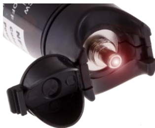
Fig. 2 Adaptor of visual fault locator
