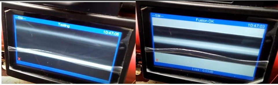
Fig. 9 Display unit shows the splicing operation going inside the fusion splice machine
